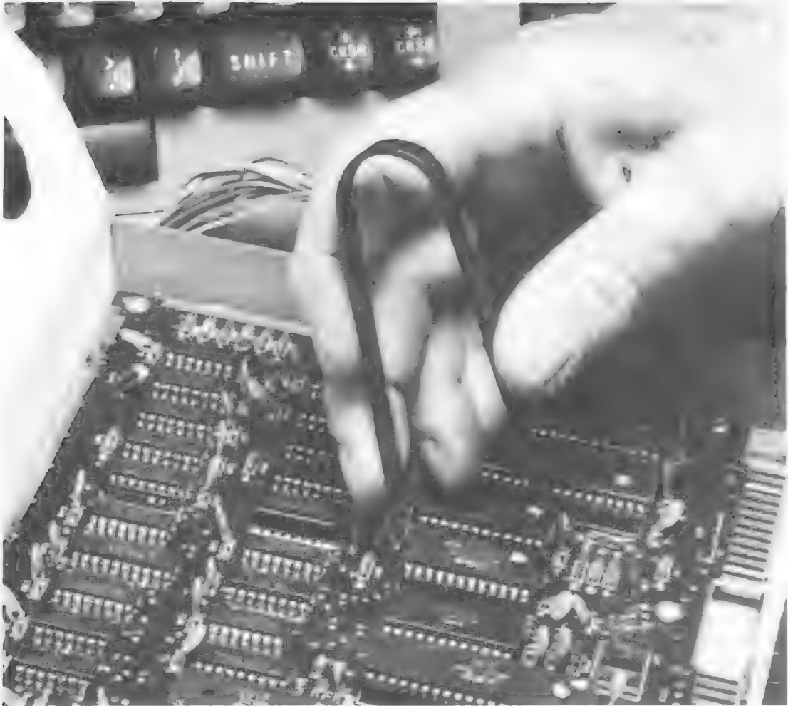
Fig. 4-10. The chip extractor is the safest way to remove chips.
